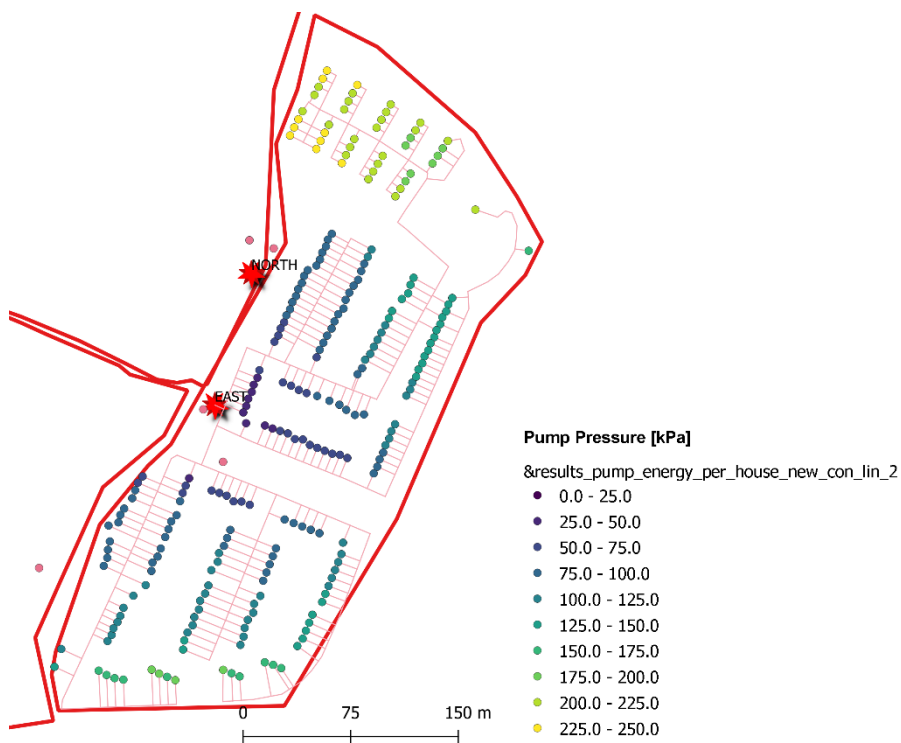
Figure 4.4 House connection pump pressure
