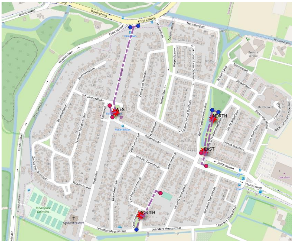
Figure 5.1 Connection of ATES wells to heat exchangers.
